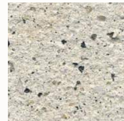
Stone seating High Performance Concrete: Pietre-di-marmo (PDM) granite, sandblasted surface id created
