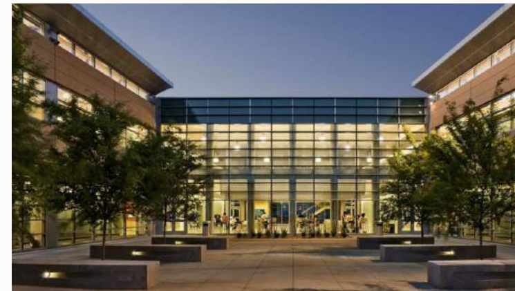
Building wall mounted cut-off luminaires placed at either side of the plaza provide general lighting while the steplights are placed as markers along the bench.
