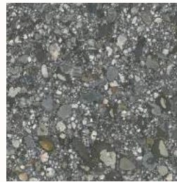
Cast In Place Concrete, or pavers Light Grey Integral Color; exposed aggregate through routing / sandblasting (Trademark) Acacia Square Hardscape
